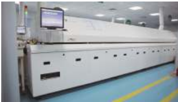
12 zones Dual Rail SMT Reflow Oven KTR-1200D/2 sets
